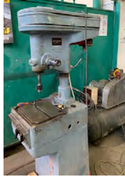
Figure 2. G13 drilling machine used for FricRiv
