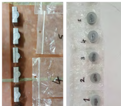
Fig 9. Specimens after cutting and specimens embedded
