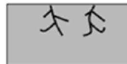
Stress corrosion cracking
