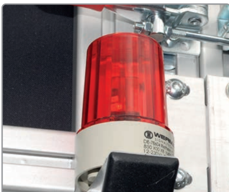
Warning lamp for signaling the operating mode.
