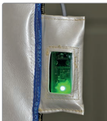
Status LED signals the correct integration in the safety circuit.
