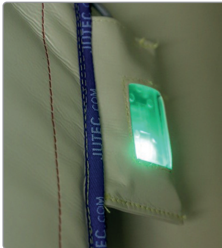
Status LED green - safety circuit closed.
