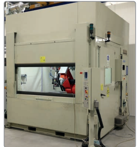
Robot cell, designed for low laser output. Thanks to the active laser protection system from JUTEC, it can now also be used for extremely high laser outputs and automated operation.
