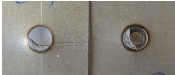
Figure 25. Partial plug failure mode in sample C3 of C-T test samples.
