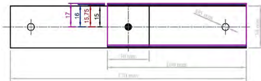
Figure 8. Tensile-shear parallel misalignment deviation sample geometry drawing.
