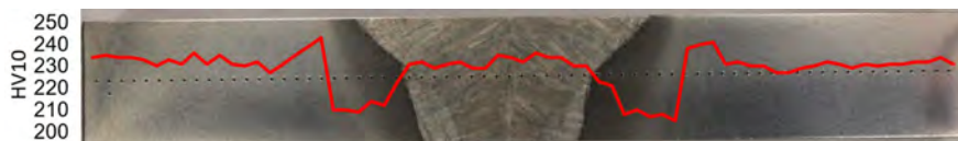
Figure 2. Macro image and hardness distribution on the Gleeble specimen
