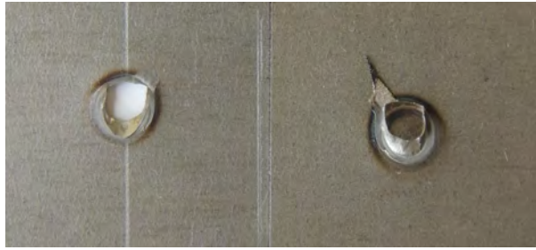
Figure 30. Expulsion failure mode after T-S testing trials.
