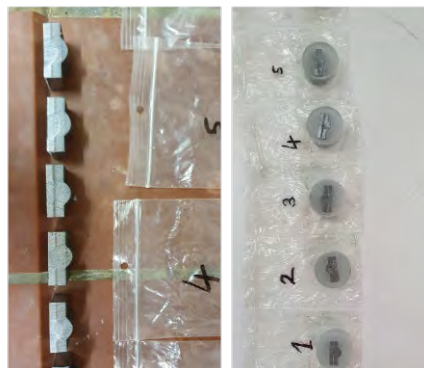
Figure 9. Specimens after cutting and specimens embedded
