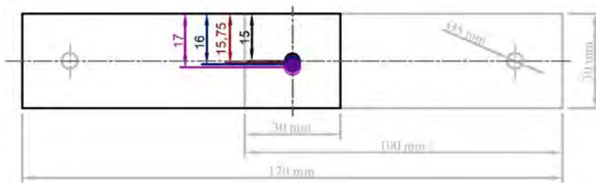
Figure 9. Tensile-shear spot weld displacement deviation sample geometry drawing.
