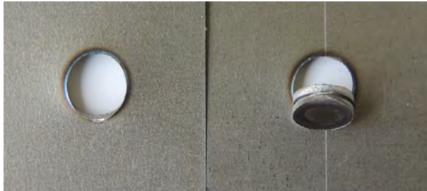
Figure 27. Plug failure mode in sample T10 of T-S test samples.
