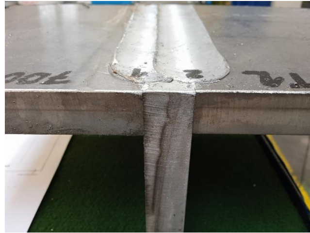
T joint 20 mm thickness – AW 6082/AW6082, two variants
